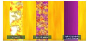
Simulated IR view of process tubes
