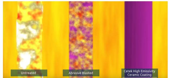
Simulated IR view of process tubes
