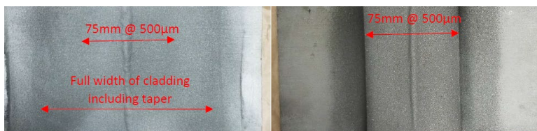
Test section edge procedure: 25mm taper (left) and 30° bevel 1mm (right)
